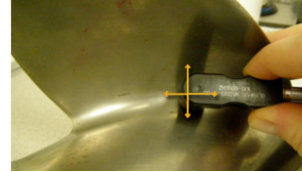
Example of scanning a propeller with eddy current testing
